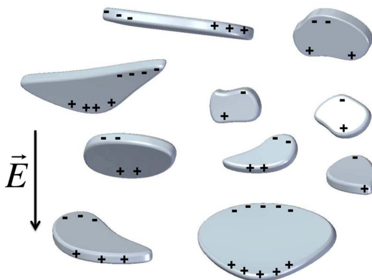
Figure 6. Scheme of the induced dipoles under electric field originated by the nanoparticles dispersed into the matrix. [Color figure can be viewed in the online issue, which is available at wileyonlinelibrary.com .]
